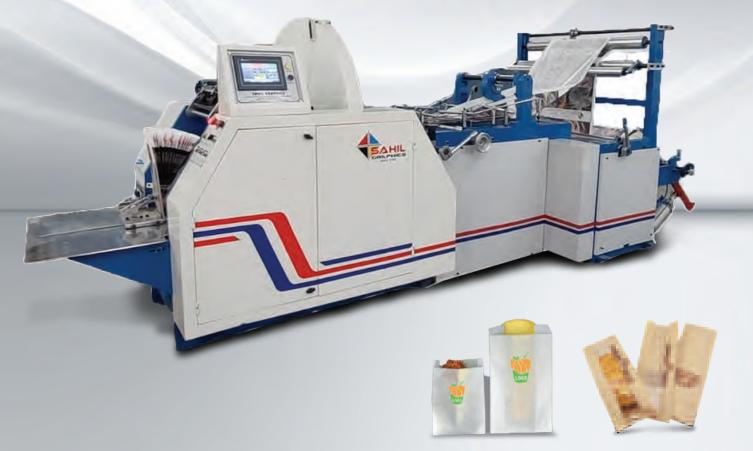
A new range of Grocery Bag Making Machine with an additional feature of servo motor so length of the bag can be changed with the help of touch screen and also pre-printed rolls can now be cut as per the desired job with High Precision Photocell Sensor.
