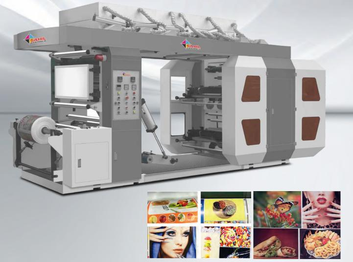
Stack type Four Colour High Speed Flexographic Printing Machine ensures easy operation, accurate colour process, particularly for long printing runs on all Rolling material multicolour/special colours printing with CMYK can be printed. This bridge type Flexographic printing machine comes with more stability and better printing quality, suitable for printing HDPE, LDPE, PP, Paper, Nonwoven Fabric etc.
