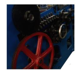
EN-8D Metal is used for gears which ensures its long life and rigidity.
